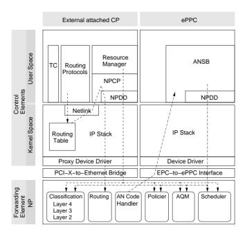
Fig. 2. Architectural overview of the implementation when the ANSB is offloaded to the ePPC.
