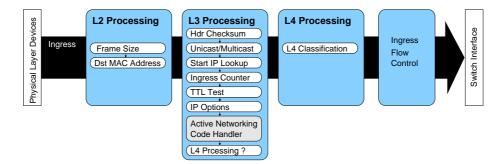
Fig. 4. Ingress data-path processing on a network processor.
