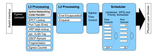
Fig. 5. Egress data-path processing on a network processor.
